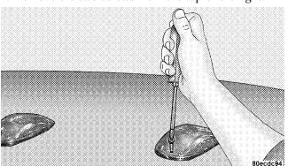
2. Rotate the socket ¼ turn and pull it from the light assembly.
